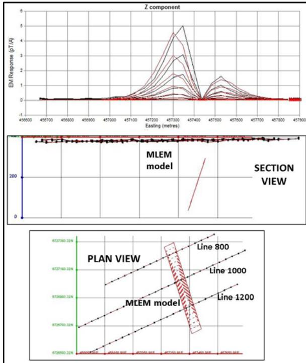
Figure 3. Northern 1000 target: Top panel – Channel 30-36 (45-220ms) in-loop MLEM response profiles (black) with MLEM model response (red). Middle & bottom panels – Section & plan views of the MLEM plate model.
