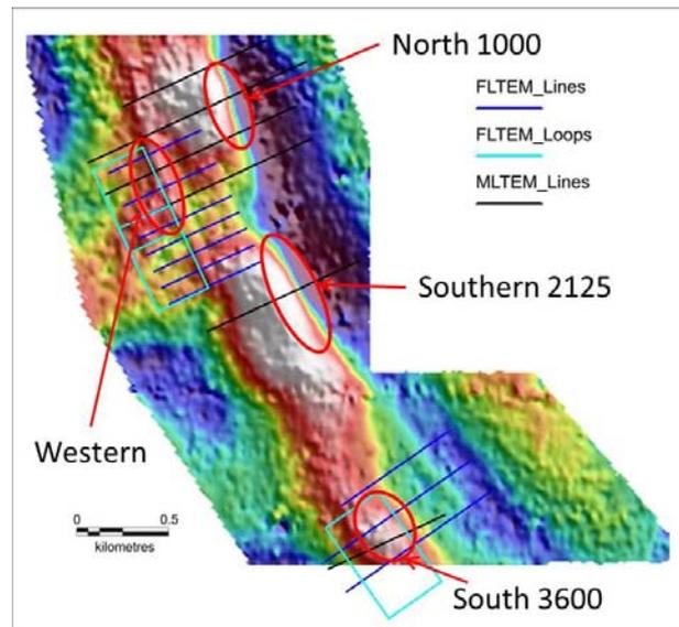
**Figure 2. Off-time channel 6 (12.5ms) GSEM grid showing the conductors identified from the GSEM data, with MLEM and FLEM line locations**
